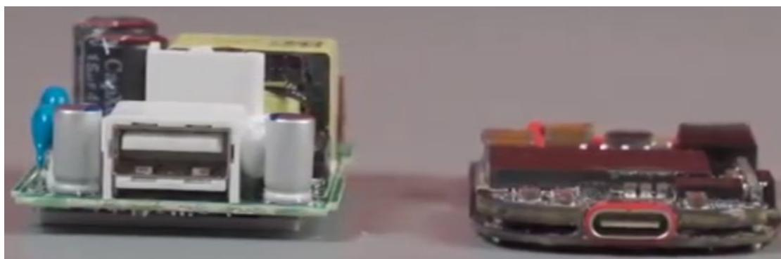
*Fig. 1: How high frequency drives smaller passive components, 50W fast-charger example. On the left, ~100 kHz traditional bobbin (22 mm high), on the right, ~500 kHz planar transformer (8 mm).*
