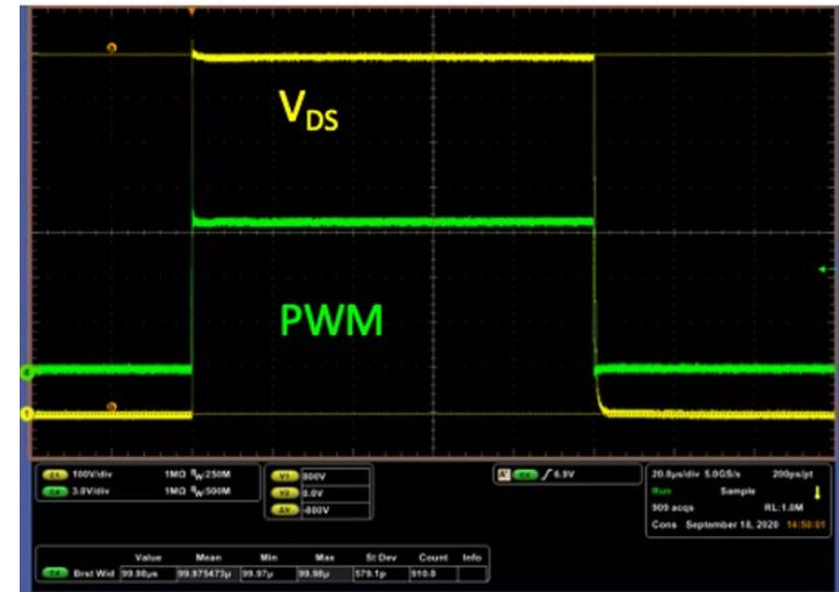
100μs pulse width, V<sub>DS</sub> = 800 V
