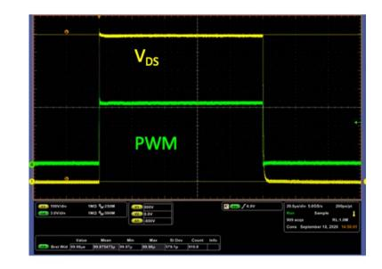
100 $\mu$ s pulse width, V<sub>DS</sub> = 800 V
