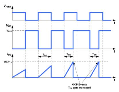
Over-Current Protection DCM Timing Diagram
