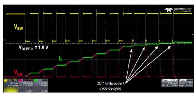
Cycle-by-cycle over current protection in CCM boost configuration
