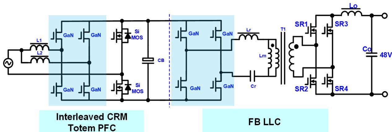
3.2 kW AC-54V converter; 650V GaNFast power ICs for MHz totem-pole PFC and MHz LLC primary with 100V GaN FETs for LLC secondary rectification.
