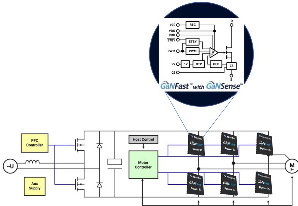
Typical Motor Drive (3-Phase) Schematic with GaNFast and GaNSense
