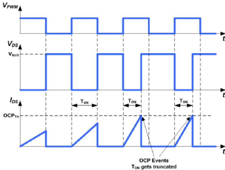
Over Current Protection DCM Timing Diagram
