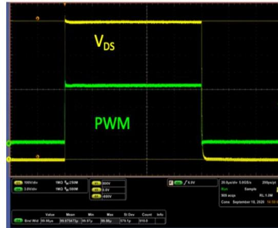
100μs pulse width,  $V_{DS} = 800$  V
