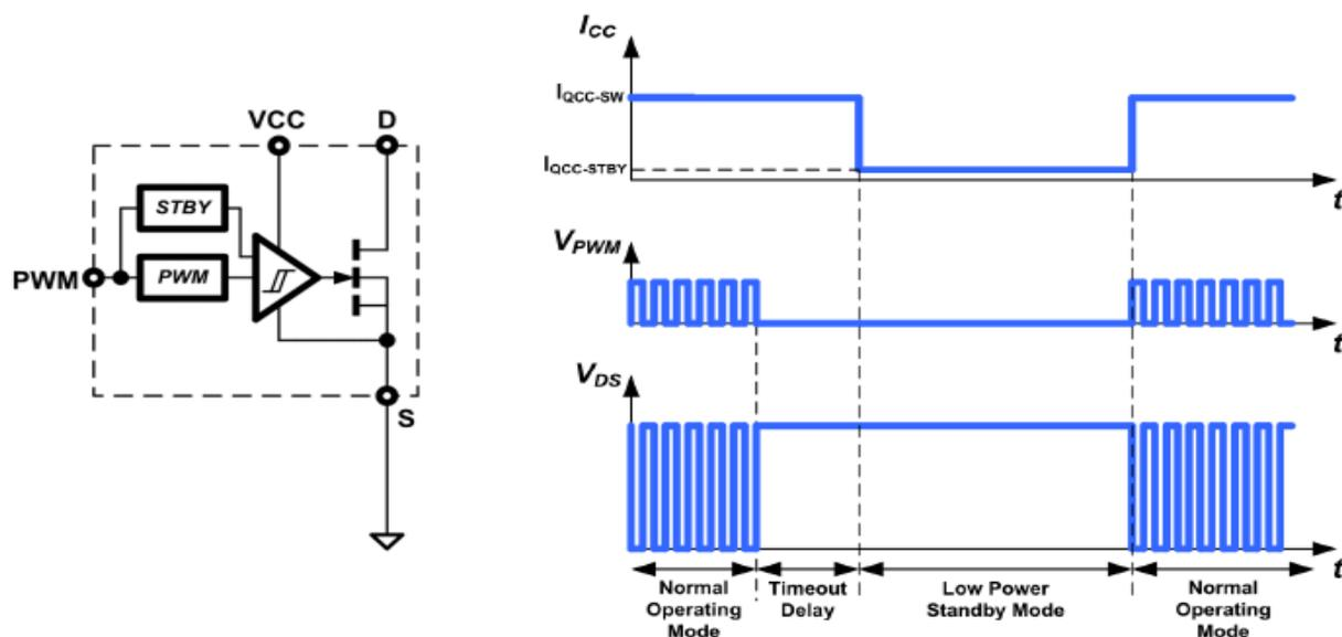
Autonomous low-power standby mode simplified circuit and timing diagram
