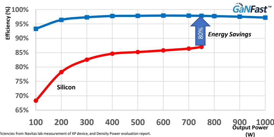
Efficiencies from Navitas lab measurement of XP device, and Density Power evaluation report.
