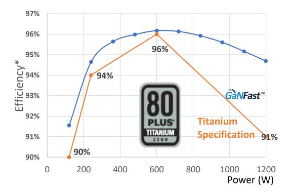
Exceeds extreme 'Titanium' grade efficiency, demanded by European Union's 'Directive 2009/125/EC, 2019 Annex', in force by January 1st, 2023. "Lower cost than silicon" – data center customer.
