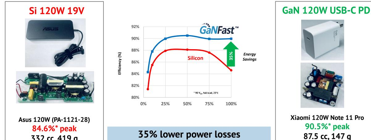
**35% lower power losses** 6% system efficiency improvement ~4x smaller system size
