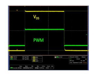
100 $\mu$ s pulse width, V<sub>DS</sub> = 800 V
