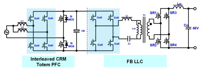
3.2 kW AC-54V converter; 650V GaNFast power ICs for MHz totem-pole PFC and MHz LLC primary with 100V GaN FETs for LLC secondary rectification.
