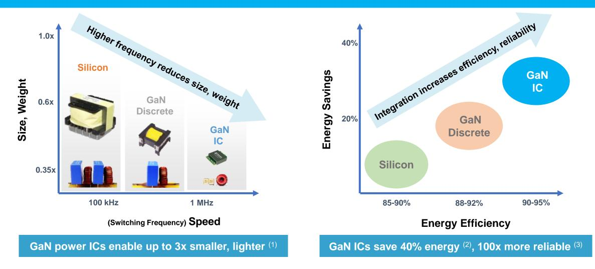
(1) Based on Navitas measurements of GaN-based chargers compared to Si-based chargers with the same output power.
