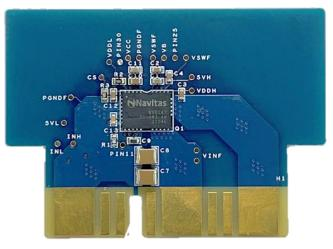
1x GaN Power IC +14 components 1/2 the Components 1/3 the Area
