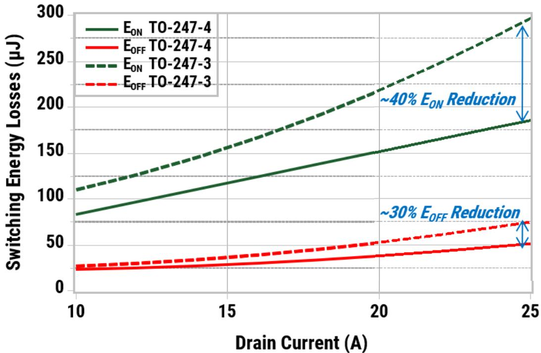
Figure 4 - Switching Loss Comparison between 3-terminal and 4-terminal MOSFET
