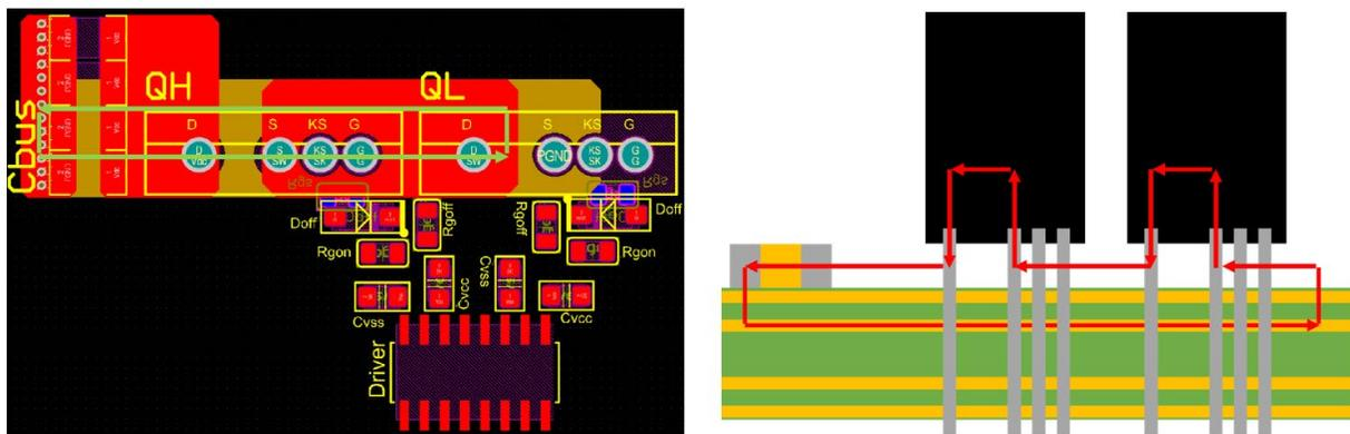
Figure 13 - Recommended power loop layout for MOSFETs in a TO-247-4 package
