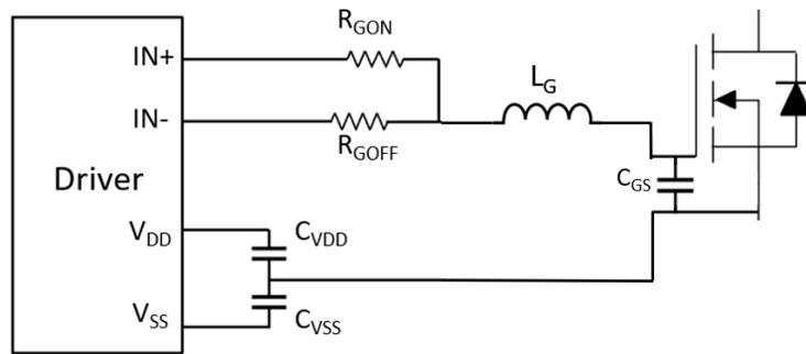
**Figure 5 - Gate Loop of SiC MOSFET**
