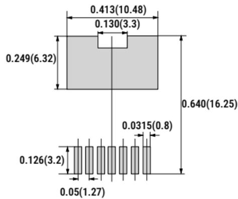
Figure 1 - Recommended Solder Pad Layout for G3R60MT07J
