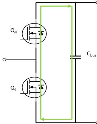
Figure 10 - High Frequency Loop of Half-Bridge Circuit
