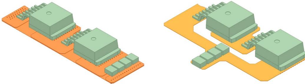
**Figure 14 - 3D models for the two PCB layouts used to extract the power loop inductance**
