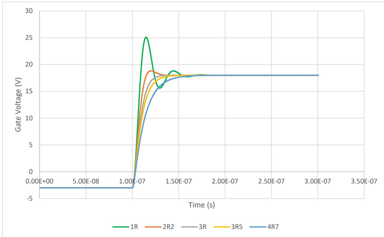
**Figure 9 - Step Response for Different  $R_g$  Values**
