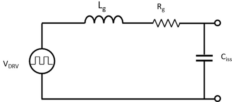
Figure 8 - Equivalent circuit of driving loop
