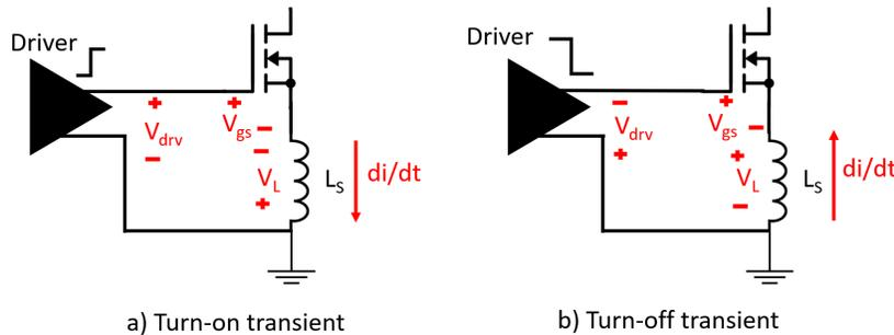
**Figure 2 - Switching Transitions in a 3 Terminal MOSFET**
