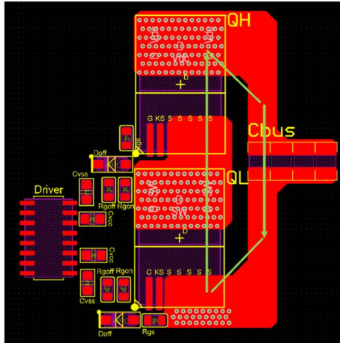
Figure 12 - Horizontal High Frequency Loop
