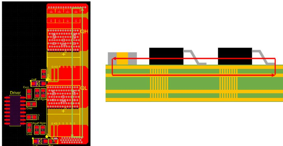
Figure 11 - Vertical High Frequency Loop
