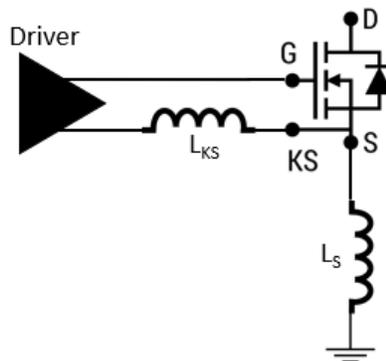
**Figure 3 - Simplified gate loop of 4-terminal MOSFET**
