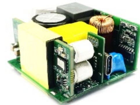
~750 kHz peak Half-Bridge GaN IC 120 W, 44 cc
