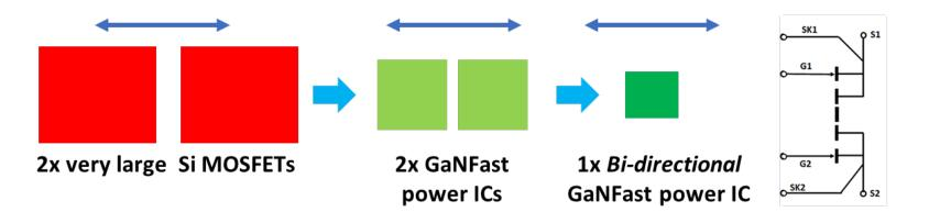
4x smaller than SiC Bi-Bi-directional FET, 3x smaller than two Uni-directional GaN, 9x smaller than Silicon
