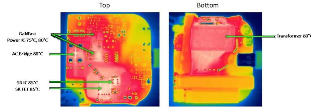
90 V<sub>AC</sub>, 45 W, 25 °C, uncased, no airflow, no thermal compound / heatsinking
