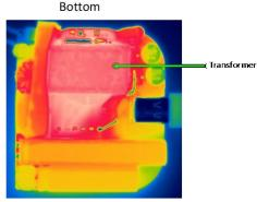
90 V<sub>AC</sub>, 45 W, 25 °C, uncased, no airflow, no thermal compound / heatsinking
