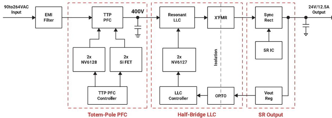
Figure 1: High-efficiency 300 W AC-DC converter
