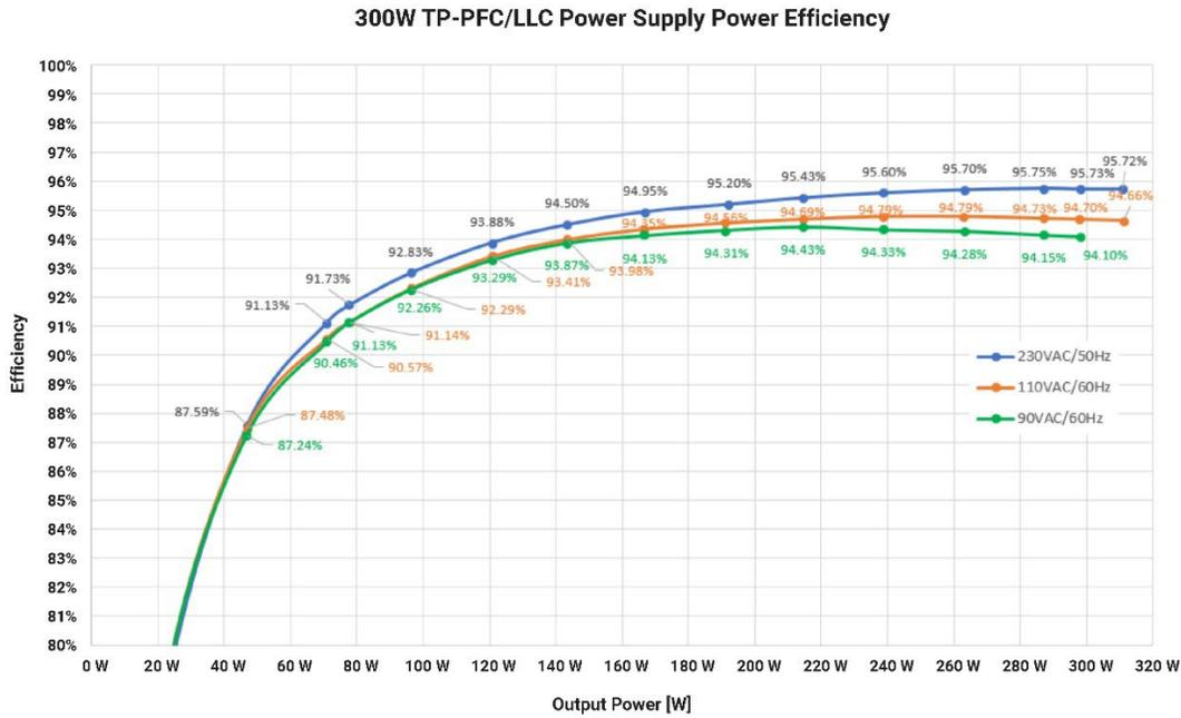
Figure 7: Power supply efficiency across the load range, operating at 90, 110, 230 V<sub>AC</sub> input
