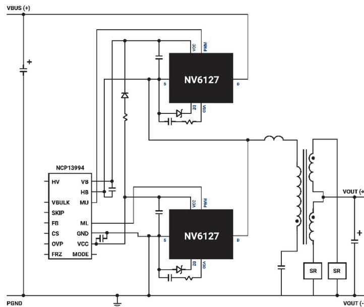
Figure 3: High-frequency half-bridge LLC resonant DC-DC converter
