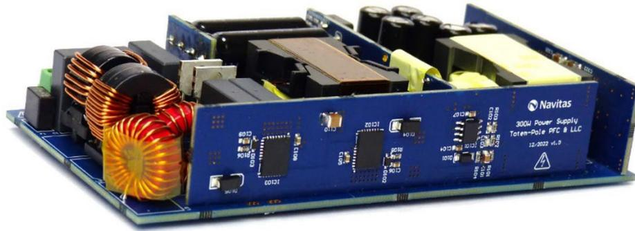
Figure 4: The prototype uncased converter with separate PFC, resonant LLC, and SR daughter cards
