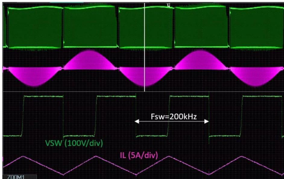
Figure 5: PFC waveforms with sinusoidal inductor current, indicating high power factor, and ZVS at  $T_{on}$  and  $T_{off}$
