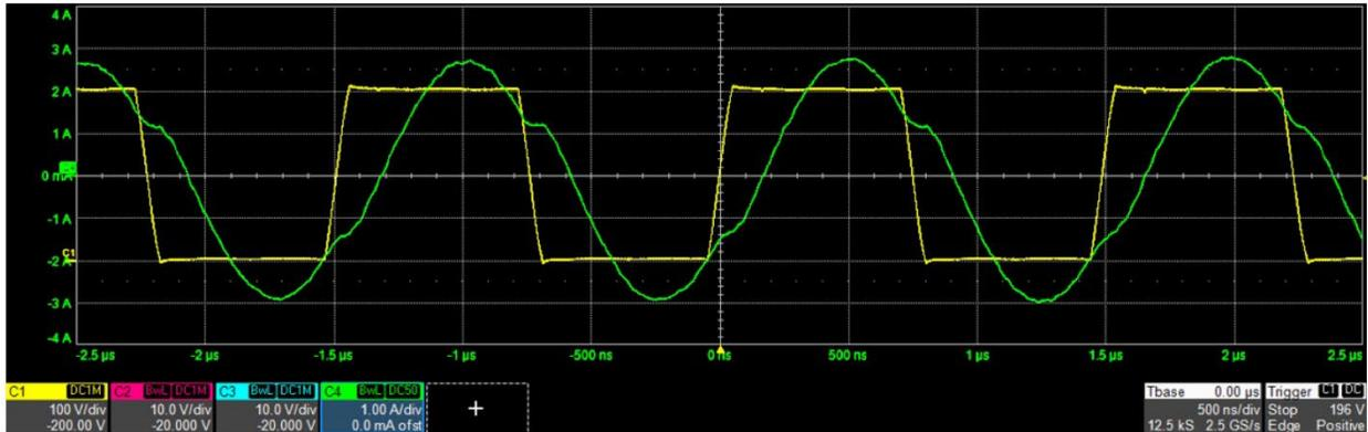
Figure 6: The LLC ZVS waveforms, showing sinusoidal current of the LLC tank circuit and smooth and clean ZVS half-bridge waveforms.
