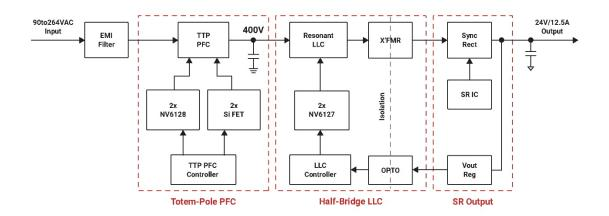
Figure 1: High-efficiency 300 W AC-DC converter
