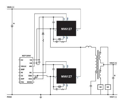
*Figure 3: High-frequency half-bridge LLC resonant DC-DC converter*
