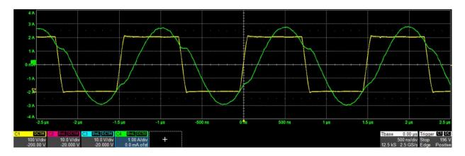
*Figure 6: The LLC ZVS waveforms, showing sinusoidal current of the LLC tank circuit and smooth and clean ZVS half-bridge waveforms.*
