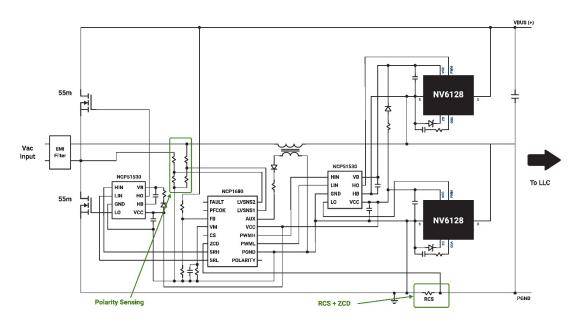
Figure 2: GTTP PFC stage designed to operate at 200 kHz
