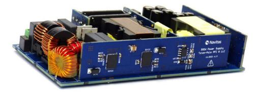
Figure 4: The prototype uncased converter with separate PFC, resonant LLC, and SR daughter cards
