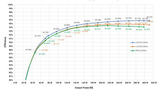
Figure 7: Power supply efficiency across the load range, operating at 90, 110, 230 V<sub>AC</sub> input
