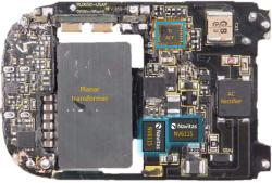
Figure 2: OPPO 50W Mini "Cookie" charger, showing high-frequency planar magnetics and elimination of electrolytic bulk capacitor.
