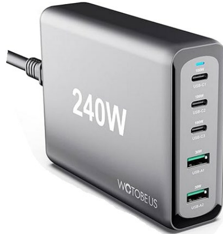
WOTOBEUS 240W-3C/2A 113 x 86 x 32 mm = 311 cc Power Density = 0.77 W/cc Efficiency = 91.3% (90Vac/100%)
