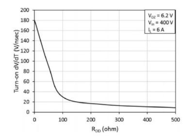
Advanced multiphase Gate Shaping for turn on dv/dt control Dv/dt controlled by programmable external Rdd
