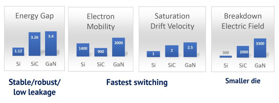
Excluding the three semiconductors  $(Ga_2O_3, Diamond, AIN)$  for which commercial devices are not available, GaN is the semiconductor with
