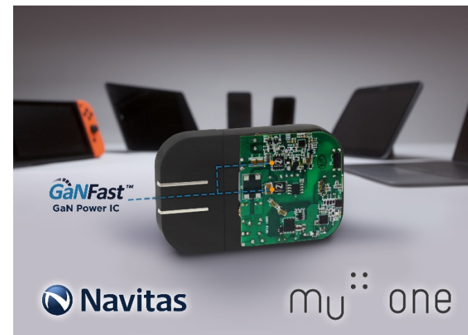
Commercial realization: Mu One 45W USB-PD 3.0, only 14 mm thin cased
