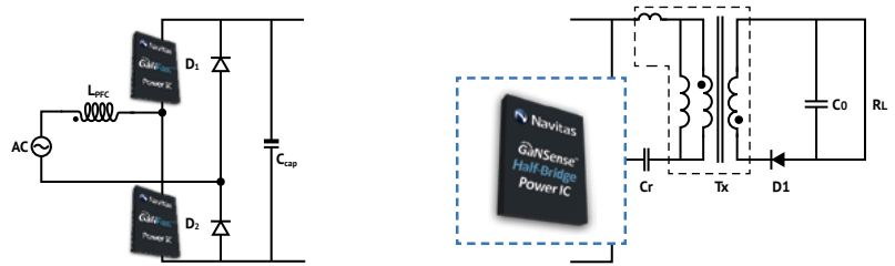
AC-DC Converter (Totem Pole + LLC + SR) using GaNSense Half-Bridge ICs
