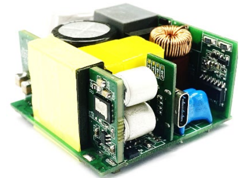
~750 kHz peak Half-Bridge GaN IC 120 W, 44 cc
