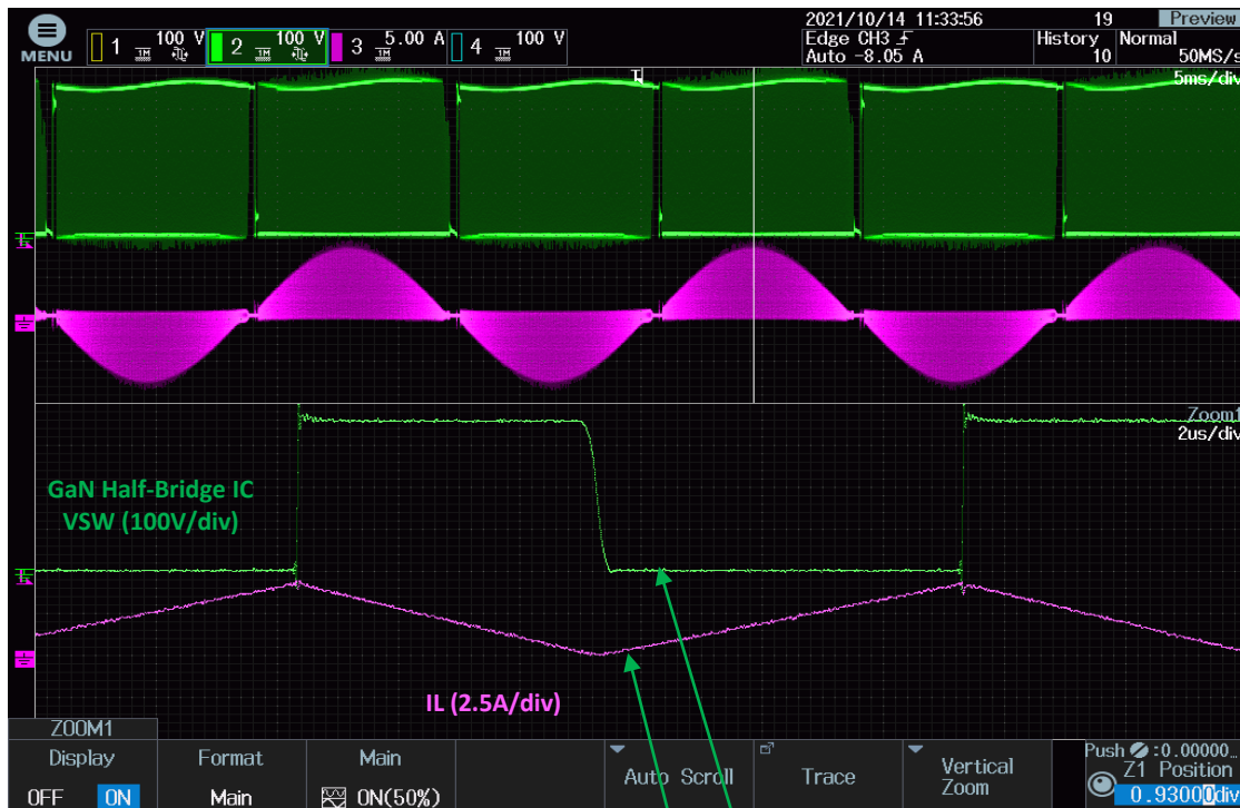
Boost Circuit Waveforms ( V_{IN} = 115 V_{AC} , P_{OUT} = 140 W )
