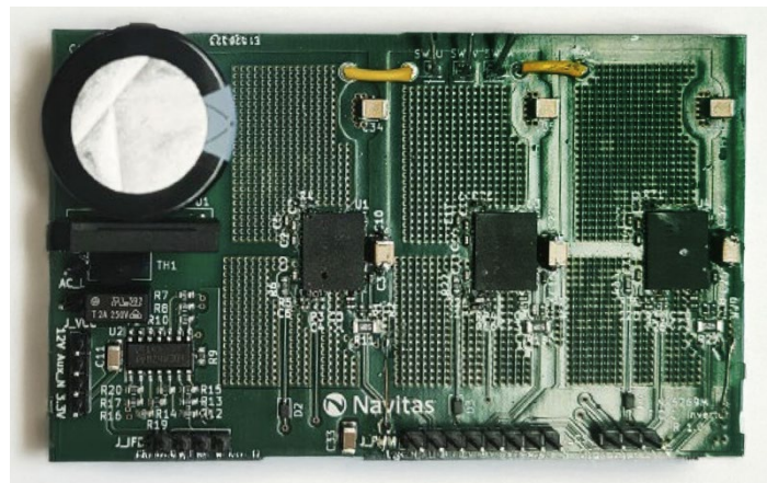
Figure 2: GaN power ICs allow a smaller DC link capacitor and heatsink-free design
