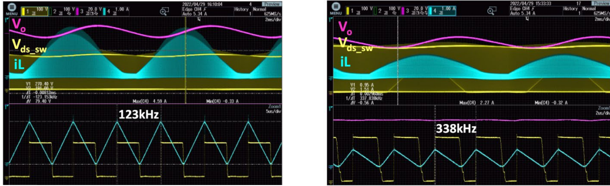
Figure 6: Boost PFC switching waveforms during full load conditions, 115 V AC input (left), 230 V AC input (right), I_L =blue (1 A/div), V_{DS} =yellow (100 V/div)
