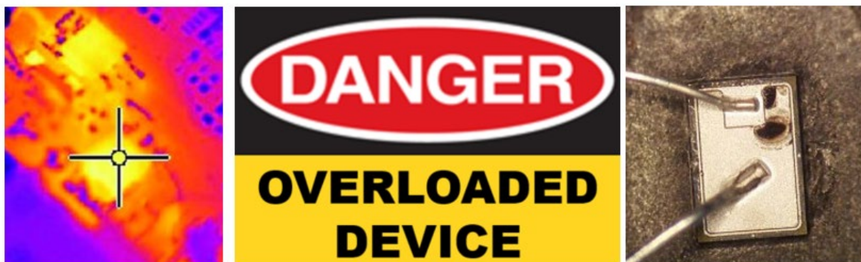
Figure 1. Device overload causes high temperatures and destruction.
