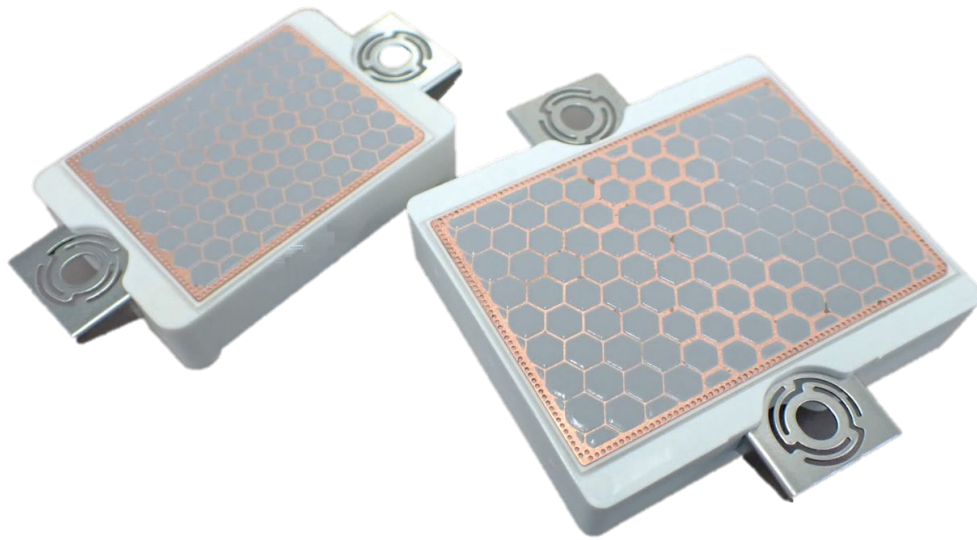
Figure 9. SiCPAK™ G module (left) and SiCPAK™ F module (right) with TIM layers pre-applied
