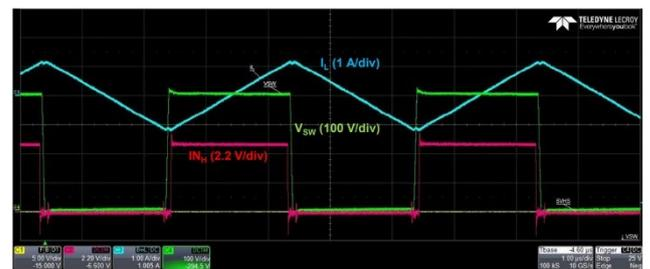
Fig. 5 Soft switching waveform of the half-bridge GaN power IC
