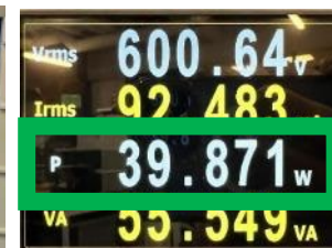
T-A PG 40 W system loss -30% SiC loss
