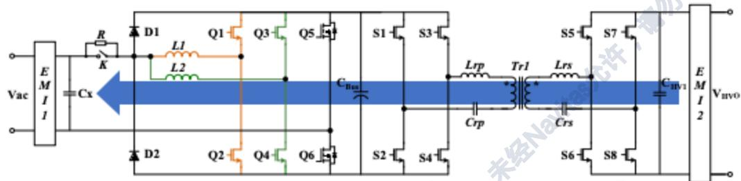
280Vbat input, 220Vac output,  $f_{s\_DC/AC} = 100\text{kHz}$ ,  $f_{s\_D2D}$
