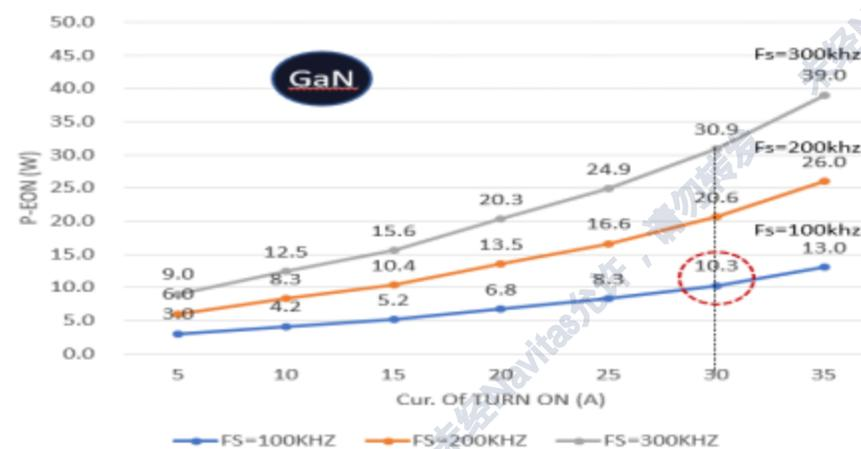
■ If the max. Eon loss is 15W@30A, the max. switching frequency can be designed at about 100kHz.
