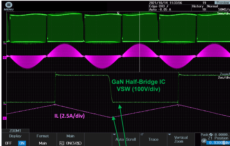
Boost Circuit Waveforms ( V_{in}=115VAC , P_o=140W )
