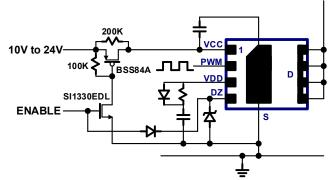
Fig. 22. Standby mode Vcc cut-off circuit
