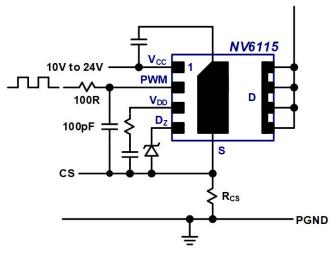
Fig. 24. Current sensing circuit
