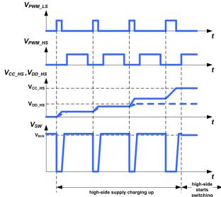
Fig. 20. ACF half-bridge start-up timing diagram
