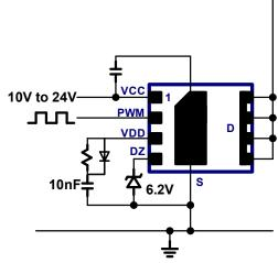
Fig. 18. Quick start-up circuit
