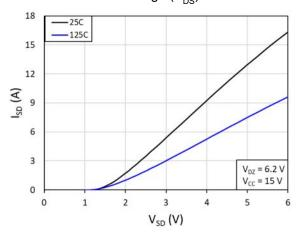
Fig. 5. Source-to-drain reverse conduction voltage
