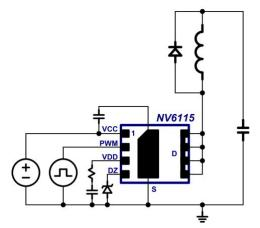
Fig. 1. Inductive switching circuit
