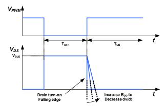
Fig. 23. Turn-on dV/dt slew rate control
