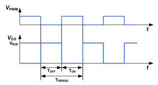
Fig. 21. Normal operating mode timing diagram
