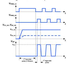
Fig. 19. LLC half-bridge start-up timing diagram
