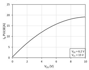
Fig. 3. Pulsed Drain current (I  $_{\rm D}$  PULSE) vs. drain-to-source voltage ( $V_{DS}$ ) at T = 25 °C
