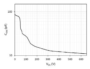
Fig. 9. Output capacitance ( $C_{\rm OSS}$ ) vs. drain-to-source voltage (V<sub>DS</sub>)
