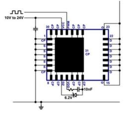
Fig. 18. Start-up circuit
