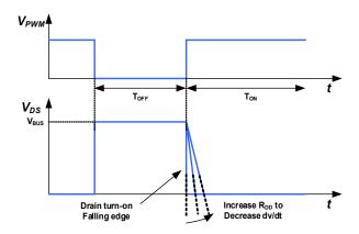
Fig. 23. Turn-on dV/dt slew rate control
