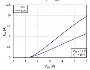
Fig. 5. Source-to-drain reverse conduction voltage
