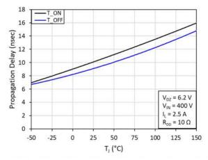
Fig. 14. Propagation delay ( $T_{\rm ON}$  and  $T_{\rm OFF}$ ) vs. junction temperature(T<sub>1</sub>)
