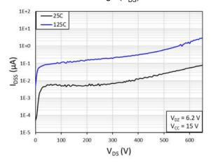
Fig. 6. Drain-to-source leakage current ( $I_{DSS}$ ) vs. drain-to-source voltage (V<sub>DS</sub>)
