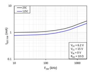
Fig. 12.  $V_{CC}$  operating current ( $I_{QCC-SW}$ ) vs. operating frequency (F<sub>SW</sub>)
