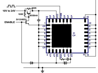
Fig. 22. Standby mode V<sub>CC</sub> cut-off circuit
