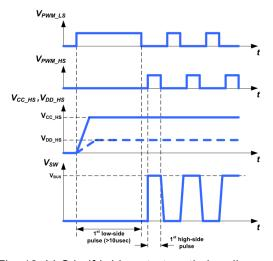
Fig. 19. LLC half-bridge start-up timing diagram
