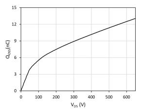
Fig. 11. Charge stored in output capacitance (Q<sub>OSS</sub>) vs. drain-to-source voltage (V<sub>DS</sub>)
