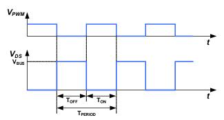
Fig. 21. Normal operating mode timing diagram
