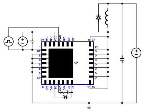
Fig. 1. Inductive switching circuit
