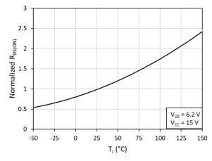
Fig. 8. Normalized on-resistance ( $R_{\text{DS}(\text{ON})}$ ) vs. junction temperature (T<sub>i</sub>)
