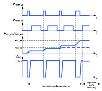
Fig. 20. ACF half-bridge start-up timing diagram
