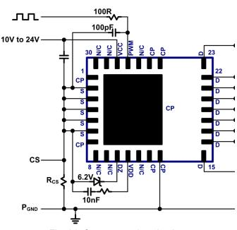
Fig. 24. Current sensing circuit
