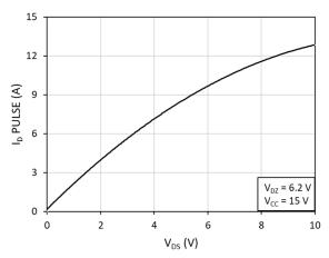
Fig. 4. Pulsed Drain current (I<sub>D</sub> PULSE) vs. drain-to-source voltage ( $V_{\rm DS}$ ) at T = 125 °C
