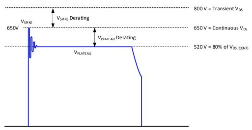
Fig. 27 QR flyback drain-to-source voltage stress diagram
