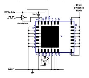
Fig. 22. SK pin connections
