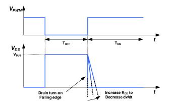
Fig. 21. Turn-on dV/dt slew rate control
