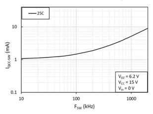
Fig. 12.  $V_{CC}$  operating current ( $I_{QCC-SW}$ ) vs. operating frequency ( $F_{SW}$ )
