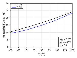
Fig. 14. Propagation delay (T<sub>ON</sub> and T<sub>OFF</sub>) vs. junction temperature(T<sub>i</sub>)
