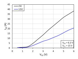
Fig. 5. Source-to-drain reverse conduction voltage
