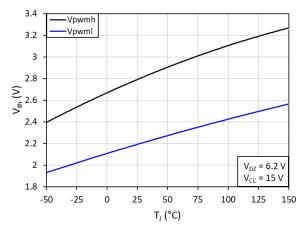
Fig. 7. V<sub>PWMH</sub> and V<sub>PWML</sub> vs. junction temperature(T<sub>i</sub>)
