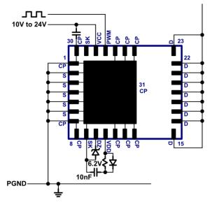
Fig. 18. Start-up circuit
