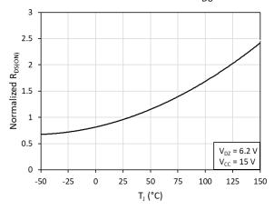
Fig. 8. Normalized on-resistance (R<sub>DS(ON)</sub>) vs. junction temperature (T<sub>1</sub>)
