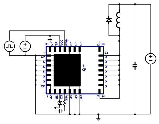
Fig. 1. Inductive switching circuit
