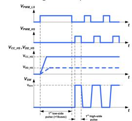
Fig. 19. LLC half-bridge start-up timing diagram
