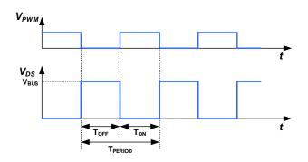
Fig. 20. Normal operating mode timing diagram
