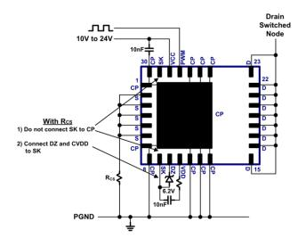
Fig. 24 NV6128 with R<sub>cs</sub> is not directly compatible with NV6127 connections
