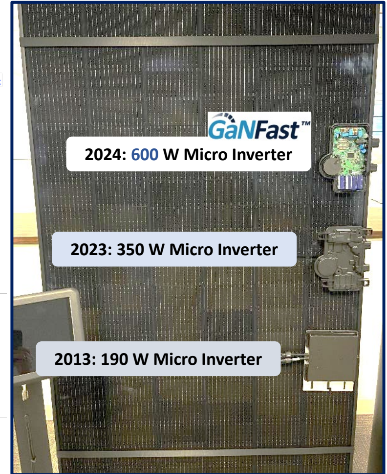
Micro Inverter with 2x Bi-Directional GaN:
