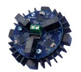
Navitas 300W 3-phase Platform for Inverter-Motor Integration
