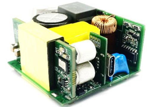
~750 kHz peak Half-Bridge GaN IC 120 W, 44 cc
