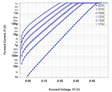
Figure 2: Low current forward I-V characteristics for 10 A SiC MPS diode.
