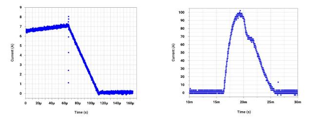
Figure 5: (a) Avalanche testing and (b) surge current characteristic
