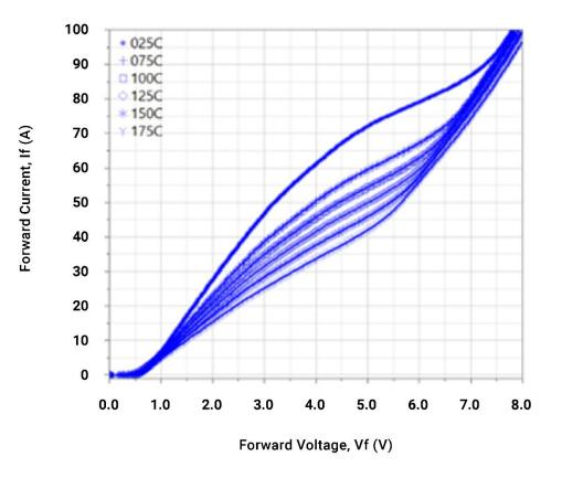
Figure 3: High-current forward-IV characteristics from 25°C to 175°C.
