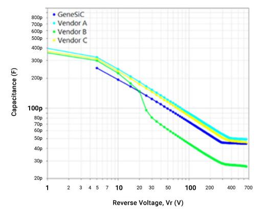
Figure 4: C-V curves for Navitas and competitor SiC MPS diodes.
