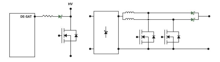
Figure 6: MPS diodes in desaturation detection circuit and interleaved PFC circuit
