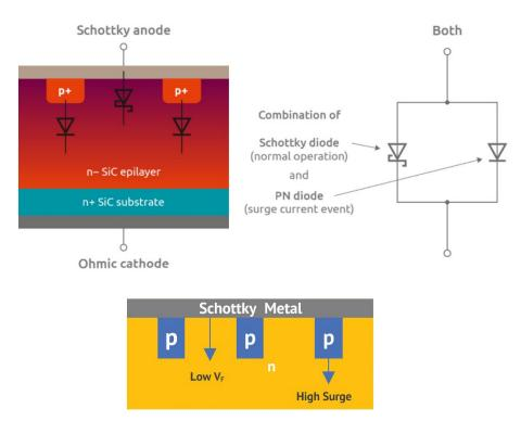
Figure 1: MPS combines PiN and Schottky diode attributes.
