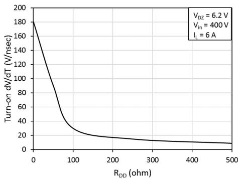
Fig. 5a:  $R_{DD}$  configuration and turn-on switching node  $dV/dt$  control.
