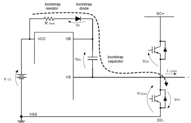
Fig. 6: Bootstrap power supply circuit implementation with discrete devices.
