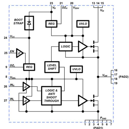
Fig. 7: Monolithically integrated GaN half bridge with high and low side driver, bootstrap and level shifter circuitry.
