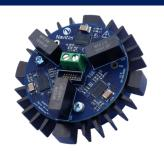
GaN-Based 300W 3-phase Platform for Inverter-Motor Integration
