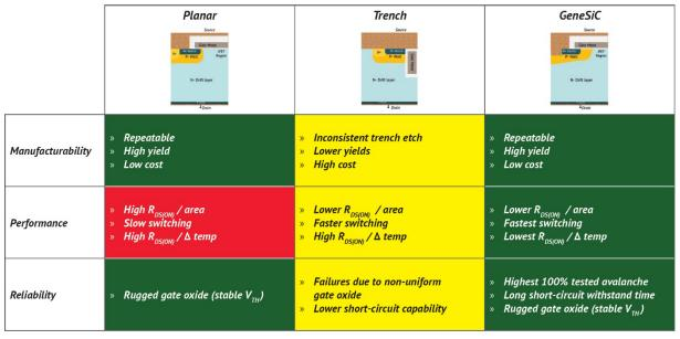
Table 1: Planar, trench, and trench-assisted planar comparison.
