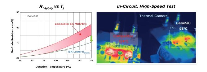
Figure 1a. Lower R<sub>DS(ON)</sub> temperature coefficient of GeneSiC MOSFETs. Figure 1b. Operating temperature reduced by 25°C.
