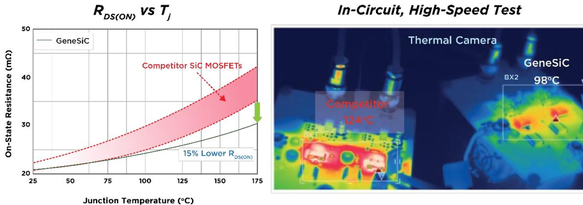
Figure 1a. Lower  $R_{DS(ON)}$  temperature coefficient of GeneSiC MOSFETs.
