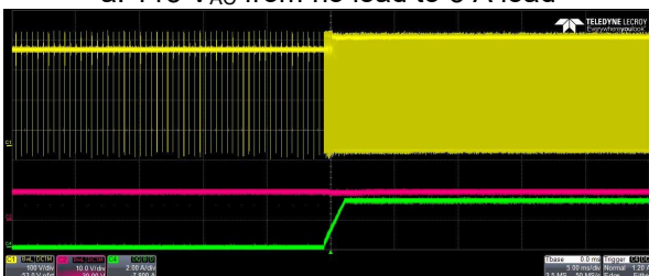
c: 230 V AC from no load to 3 A load
