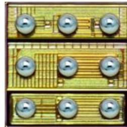
EPC2107 devices are supplied only in passivated die form with solder balls
