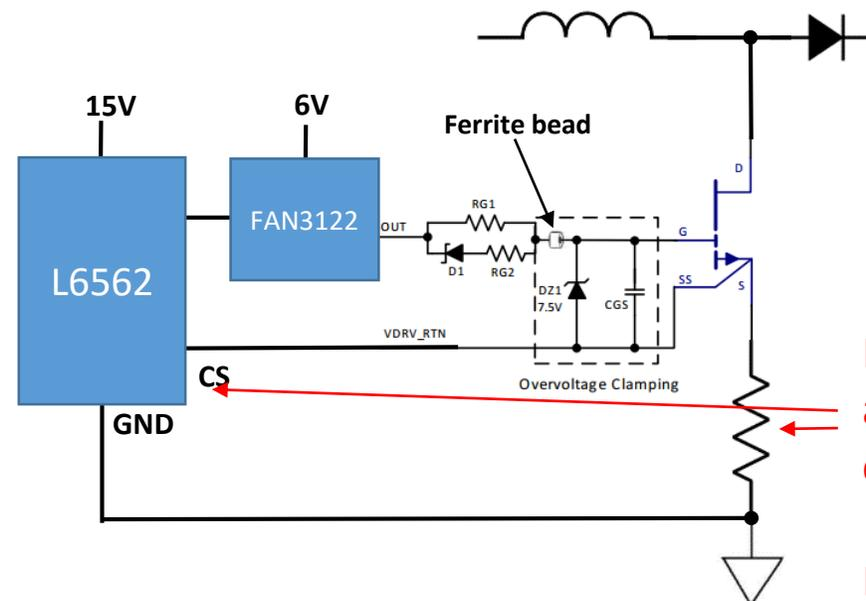
PFC IC needs sense resistor and source connection for current sensing
