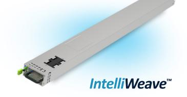
Navitas' OCP 12 kW solution adopts a 3-phase interleaved TP-PFC topology that uses IntelliWeave digital control to provide CCM or CrCM switching techniques, powered by Gen 3-Fast SiC MOSFETs, and a 3-phase interleaved FB LLC topology using high-power GaNSafe ICs.
