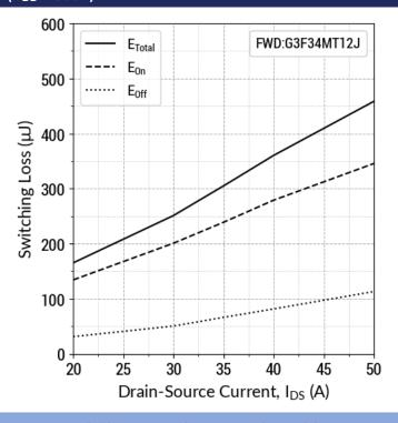
$T_i = 25$ °C;  $V_{GS} = -5/+18V$ ;  $R_{G(ext)} = 4 \Omega$ ;  $L = 40.0 \mu H$
