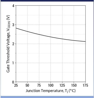
$V_{GS(th)} = f(T_j); V_{DS} = V_{GS}; I_D = 18 \text{ mA}$
