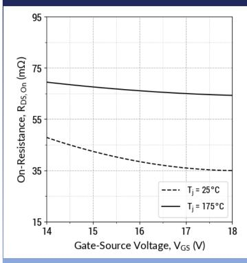
$R_{DS(ON)} = f(T_j, V_{GS}); t_P = 50 \mu s; I_D = 26 A$
