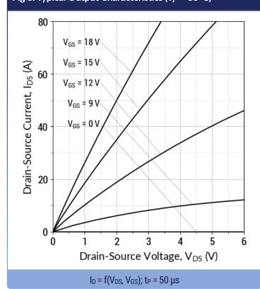
Fig 4: Typical Output Characteristics (V<sub>GS</sub> = 18 V)
