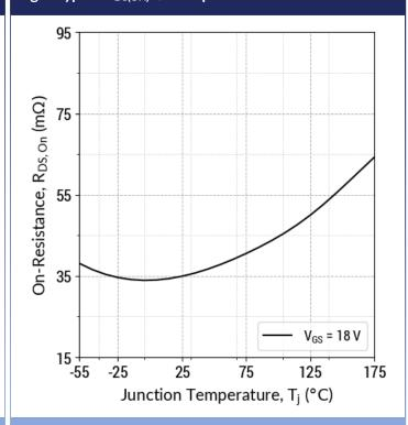
$R_{DS(ON)} = f(T_j, V_{GS}); t_P = 50 \mu s; l_D = 26 A$
