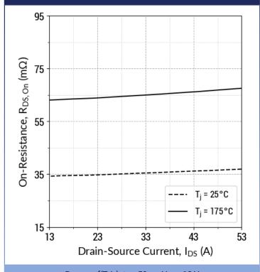
$R_{DS(ON)} = f(T_j,I_D)$ ;  $t_P = 50 \mu s$ ;  $V_{GS} = 18 \text{ V}$
