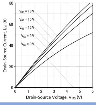
$I_D = f(V_{DS}, V_{GS}); t_P = 50 \mu s$
