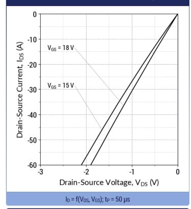
Fig 22: Typical Third Quadrant Characteristics ( $T_j = 175^{\circ}$ C)
