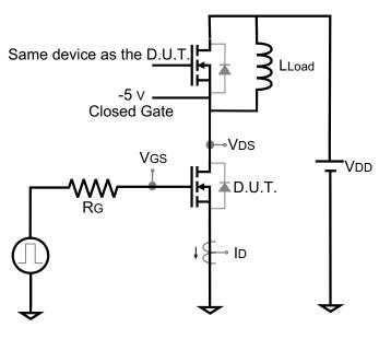
Note: Gate Charge, Switching Time and Energy Circuit
