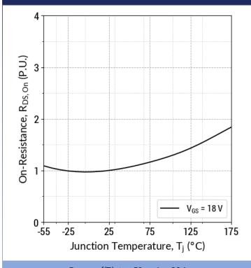
$R_{DS(ON)} = f(T_j); t_P = 50 \mu s; I_D = 26 A$
