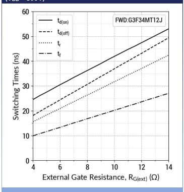
$T_i = 25$ °C;  $V_{GS} = -5/+18V$ ;  $I_{DS} = 26$  A;  $L = 40.0 \mu H$
