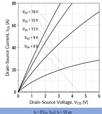
Fig 2: Typical Output Characteristics ( $T_j = 175$ °C)
