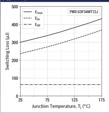
$T_i = 25$ °C;  $V_{GS} = -5/+18V$ ;  $R_{G(ext)} = 4 \Omega$ ;  $I_{DS} = 26 A$ ;  $L = 40.0 \mu H$
