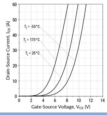
$I_D = f(V_{GS}, T_i); t_P = 100 \mu s$
