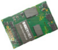
GaN 1 kW (Density Power DQB1K0F380S48) 850 kHz, 97.7% peak 58.4 x 36.8 x 14.5 mm = 31 cc 32 W/cc
