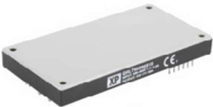
Silicon 750W (XP QHL750300S48) 200 kHz, 92% peak 116.8 x 61 x 12.7 = 90 cc 8 W/cc
