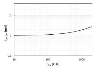
Fig. 11.  $\rm V_{\rm CC}$  operating current ( $\rm I_{\rm QCC\text{-}SW})$  vs. operating frequency (F<sub>SW</sub>)
