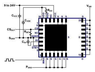
Fig. 20. IC connection diagram
