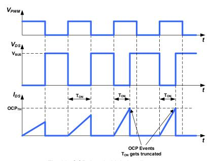
Fig. 28. OCP threshold timing diagram
