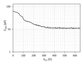
Fig. 8. Output capacitance  $(C_{OSS})$  vs. drain-to-source voltage (V<sub>DS</sub>)
