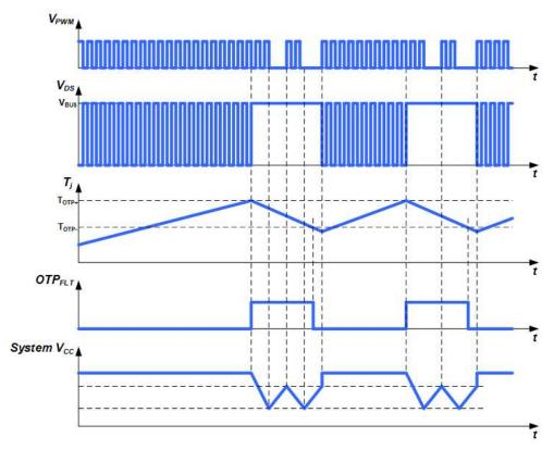
Fig. 29. OTP threshold timing diagram
