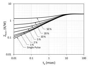
Fig. 17. Max. thermal transient impedance (Z<sub>thJC</sub>) vs. pulse width (t<sub>P</sub>)
