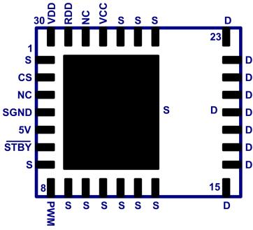
Fig. 19. Package Top View
