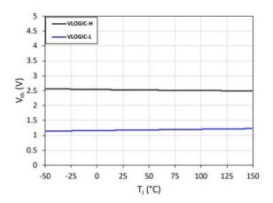
Fig. 6. VLOGIC-H and VLOGIC-L vs. junction temperature(T<sub>1</sub>)
