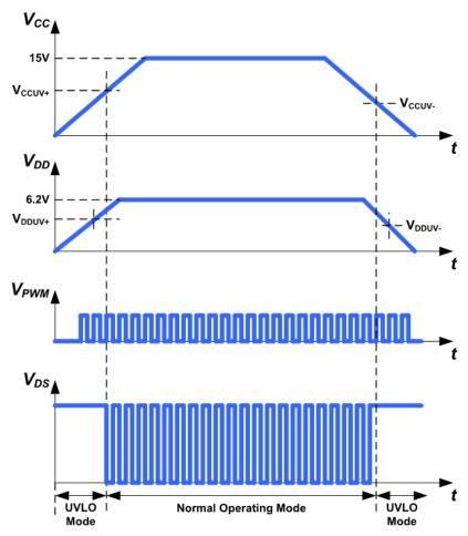
Fig. 22. UVLO Mode timing diagram
