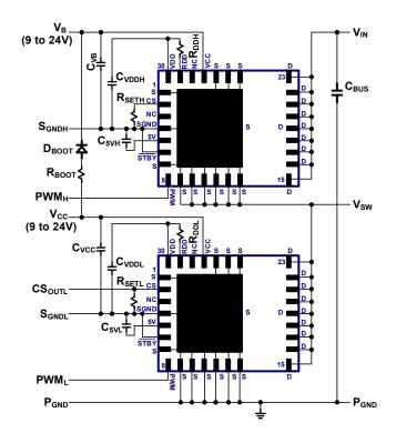
Fig. 21. Half-Bridge Configuration
