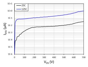
Fig. 5. Drain-to-source leakage current ( $I_{\rm DSS}$ ) vs. drain-to-source voltage (V<sub>DS</sub>)
