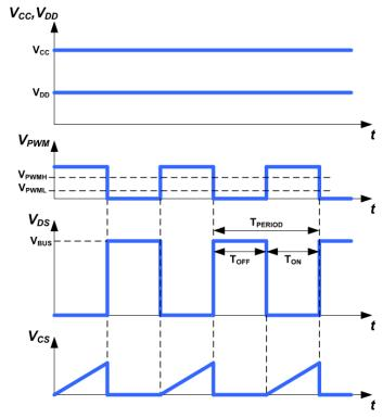
Fig. 23. Normal operating mode timing diagram
