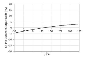
Fig. 18. CS Pin Current Output Drift vs. case temperature (T<sub>C</sub>)
