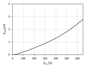
Fig. 9. Energy stored in output capacitance ( $E_{\rm OSS}$ ) vs. drain-to-source voltage (V<sub>DS</sub>)
