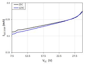
Fig. 13. VCC stand-by quiescent current (IQCC) vs. supply voltage (V<sub>CC</sub>)
