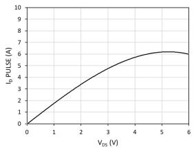
Fig. 3. Pulsed Drain current ( $I_D$  PULSE) vs. drain-to-source voltage (V<sub>DS</sub>) at T = 125 °C
