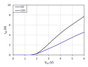
Fig. 4. Source-to-drain reverse conduction voltage
