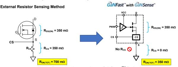
Fig. 27. External resistor sensing vs. GaNSense™ Technology
