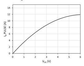
Fig. 2. Pulsed Drain current ( $I_D$  PULSE) vs. drain-to-source voltage (V<sub>DS</sub>) at T = 25 °C
