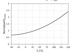
Fig. 7. Normalized on-resistance  $(R_{DS(ON)})$  vs. junction temperature (T<sub>,</sub>)
