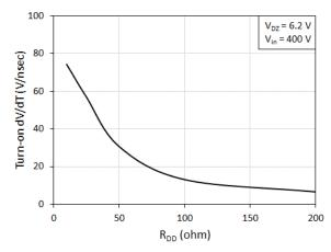
Fig. 15. Slew rate (dV/dt) vs. gate drive turn-on current set resistance (R $_{\rm DD}$ ) at T = 25  $^{\circ}$ C
