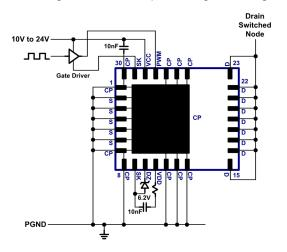
Fig. 22. SK pin connections
