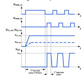
Fig. 19. LLC half-bridge start-up timing diagram
