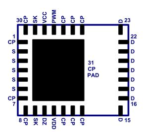
Connect CP to S or PGND in PCB layout See PCB layout section of this datasheet
