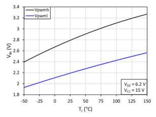
Fig. 7.  $\rm V_{PWMH}$  and  $\rm V_{PWML}$  vs. junction temperature(T<sub>1</sub>)
