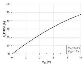
Fig. 3. Pulsed Drain current (I<sub>D</sub> PULSE) vs. drain-to-source voltage (V<sub>DS</sub>) at T = 25 °C
