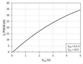
Fig. 4. Pulsed Drain current ( $I_D$  PULSE) vs. drain-to-source voltage (V<sub>DS</sub>) at T = 125 °C
