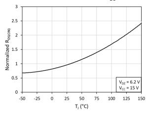
Fig. 8. Normalized on-resistance ( $R_{\text{DS(ON)}}$ ) vs. junction temperature (T<sub>i</sub>)
