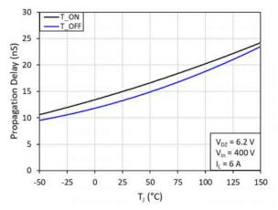
Fig. 14. Propagation delay (T $_{\rm ON}$  and T $_{\rm OFF}$ ) vs. junction temperature(T<sub>i</sub>)
