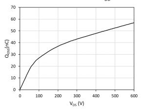
Fig. 11. Charge stored in output capacitance ( $Q_{OSS}$ ) vs. drain-to-source voltage (V<sub>DS</sub>)
