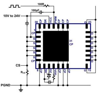
Fig. 25 Current sensing circuit
