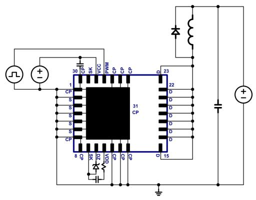
Fig. 1. Inductive switching circuit
