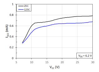
Fig. 13.  $V_{CC}$  quiescent current ( $I_{QCC}$ ) vs. supply voltage (V<sub>CC</sub>)
