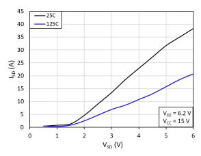
Fig. 5. Source-to-drain reverse conduction voltage
