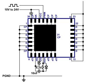
Fig. 18. Start-up circuit
