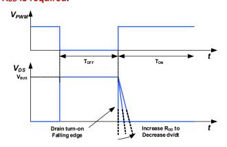
Fig. 21. Turn-on dV/dt slew rate control
