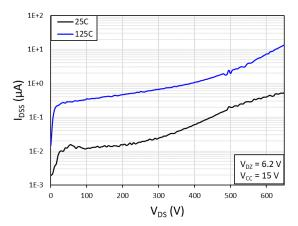
Fig. 6. Drain-to-source leakage current ( $I_{DSS}$ ) vs. drain-to-source voltage (V<sub>DS</sub>)
