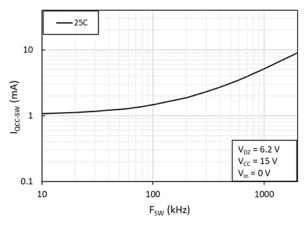
Fig. 12.  $V_{CC}$  operating current ( $I_{QCC-SW}$ ) vs. operating frequency (F<sub>SW</sub>)
