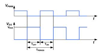
Fig. 20. Normal operating mode timing diagram
