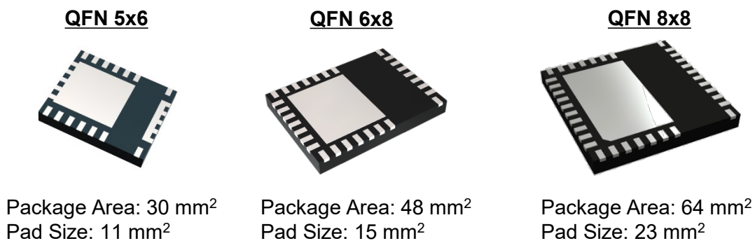
Figure 1. QFN 5x6, QFN 6x8, QFN 8x8 package types
