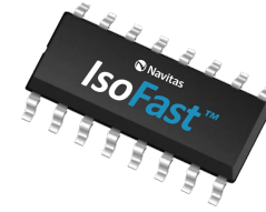
High-speed dual-channel digital Isolated GaN driver
